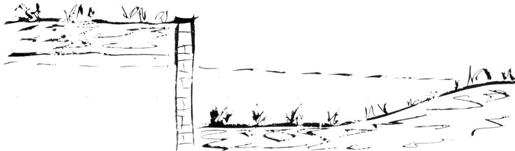
The Ha-ha is simply a sunken ditch which divides the farm pasture from the garden, yet which is only visible from a few yards away. It consists of a retaining wall constructed of brick or stone on the garden side, and a sloping bank on the pasture side.
